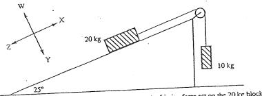
If this system of masses is at rest, in what direction does the friction force act on the 20 kg block?
