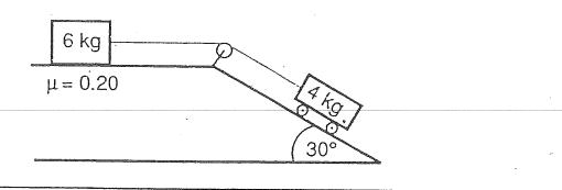
2. The above diagram shows a 6.0 kg mass on a horizontal surface connected by thread over a pulley to a 4.0 kg cart on a ramp inclined at 30°. The coefficient of friction between the horizontal surface and the 6.0 kg mass is 0.20 and the friction between the 4 kg cart and the ramp is not significant. What is the tension in the thread when the masses are accelerating? (10 marks)
