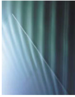
Figure 10 Waves are refracted as they cross a boundary between deep and shallow water if the boundary is at an angle.
