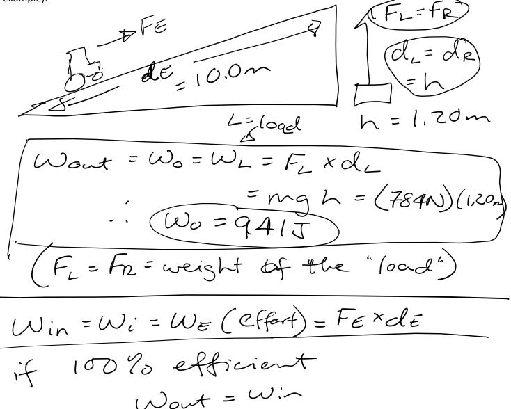
o a  $F_L \times d_L = F_E d_E$  $\frac{\partial}{\partial \sigma} F_{E} = \frac{F_{L} \times d_{c}}{d\varepsilon} = \frac{(mg \times h)}{d\varepsilon}$  $F_E = \frac{(80 kg)(9.8 N/kg)(1.2m)}{10m}$ FE = 94,1NS this is much easier than trying to lift vertically with aforce of F<sub>2</sub> = 78AN The Machine increases the distance, but reduces force, thus making work easier and safer.
